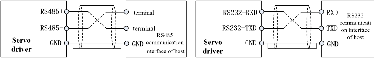
Fig. 3-13 Wiring of communication terminals
